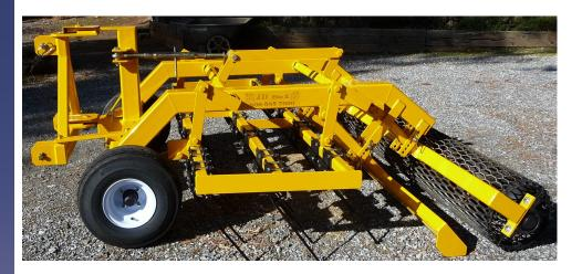
The Rudy harrow was specially designed for arenas with temperamental felt footing additives or custom sand.
