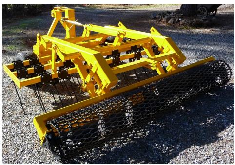
The swivel hitch allows a smooth turning radius for the greates possible access and coverage. The swivel hitch also provides a highly satisfactory relationship between the tractor and harrow by reducing negative friction on the tractor while turning. The swivel is equipped with a lock bar, which allows the operator to travel from one arena to another without uncomfortable fishtailing.
